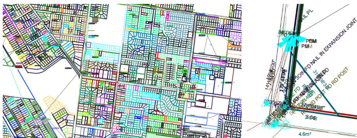
Figure 26: XBLIN imported network (left) and typical corner with multiple plan connections to marks (right).
