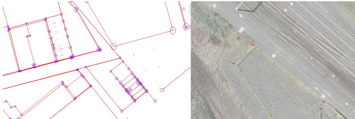
Figure 24: Error ellipses of cadastral boundaries (left) and shifts to the DCDB (right).
