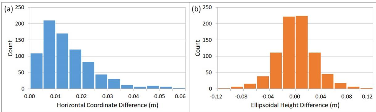
Figure 2: (a) Horizontal coordinate differences and (b) ellipsoidal height differences between multiple NRTK occupations.
