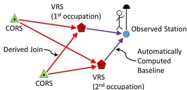
Figure 4: NRTK automatic baseline network being connected to datum via a join between each VRS and the two nearest CORS.
