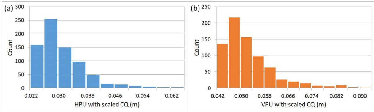
Figure 3: Calculated (a) HPU and (b) VPU for NRTK observations based on CQ output scaled by a factor of 2.1.
