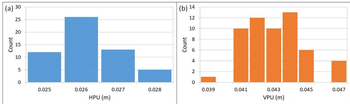
Figure 6: Calculated (a) HPU and (b) VPU for NRTK observations based on the NRTK baseline network.
