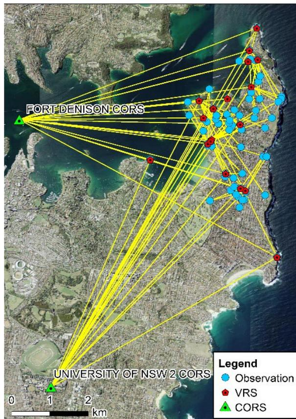
Figure 5: NRTK baseline network including the joins from each VRS to the two nearest CORS.
