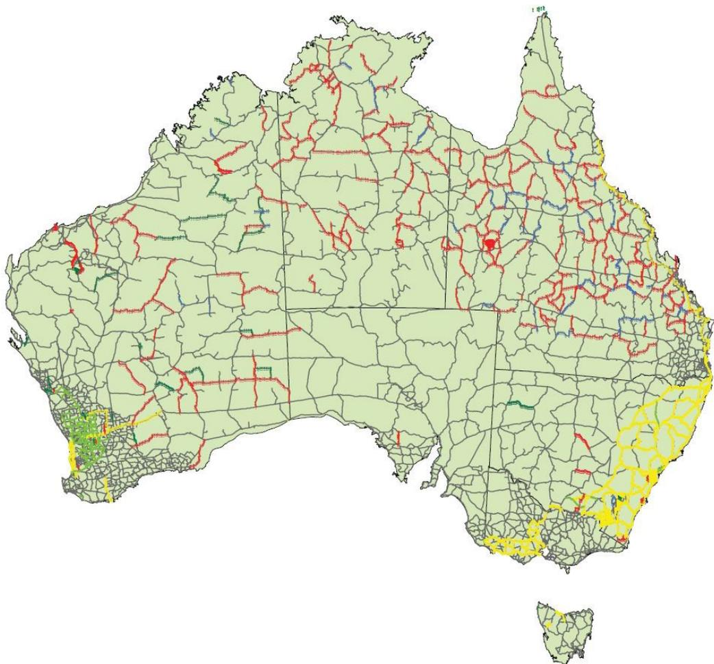
Figure 4: ANLN, showing first-order levelling sections (yellow), second-order sections (light green), third-order (fine grey), fourth-order (dark green), 1-way third-order (red) and 2-way levelling of undefined quality (blue) (Filmer et al., 2010).
