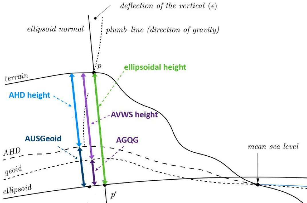
Figure 12: Converting ellipsoidal heights (green) to AHD heights (light blue) by subtracting the AUSGeoid model (dark blue) and to AVWS heights (light purple) by subtracting the AGQG model (dark purple) (ICSM, 2020b).
