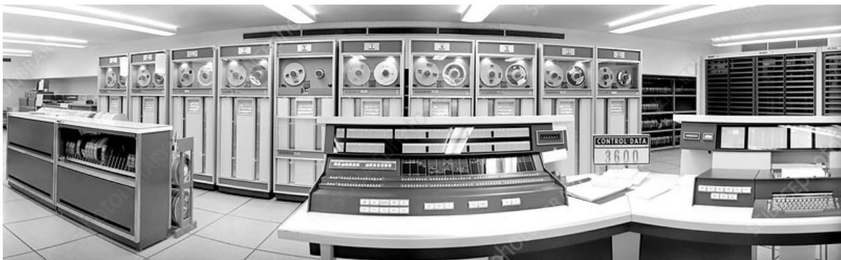
Figure 5: Control Data Corporation CDC 3600 computer used for the AHD adjustment.
