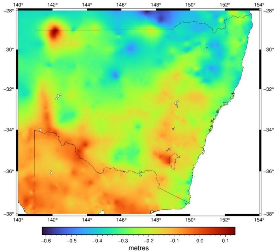
Figure 11: Differences in N values between AGQG 20201120 and AUSGeoid2020 across NSW, which is equivalent to the differences between AVWS heights and AHD heights.
