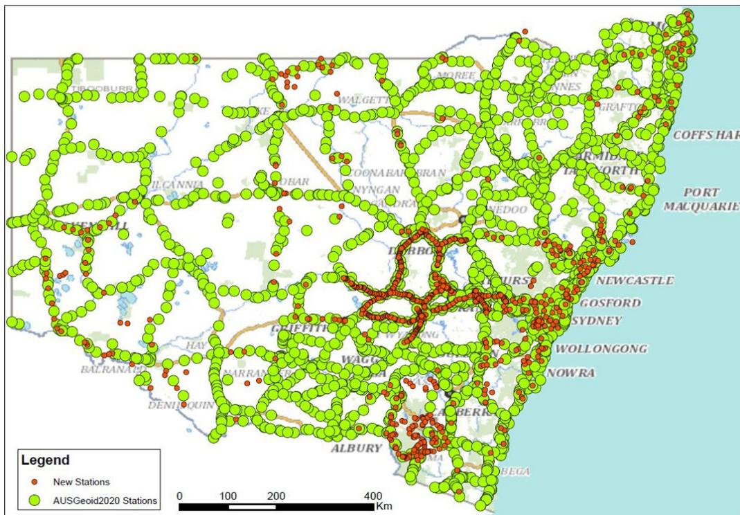
Figure 7: GNSS datasets of at least 6 hours duration on levelled marks observed by DCS Spatial Services, including those contributing to AUSGeoid2020.
