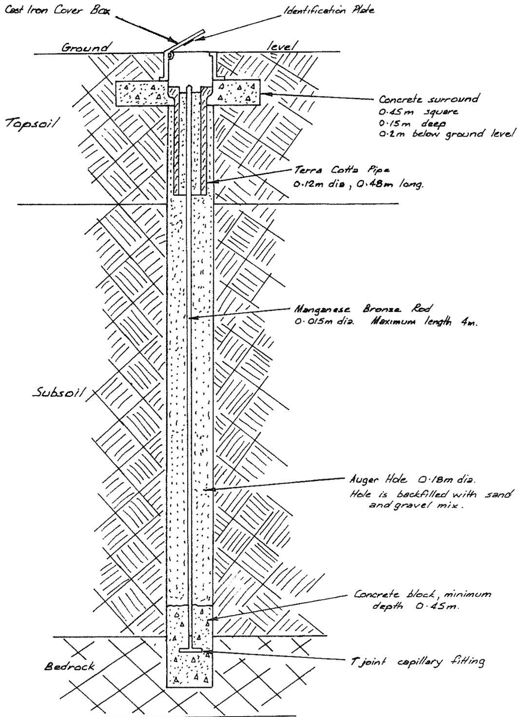
Figure 3: Fundamental Bench Mark (FBM) design (Naylor, 1976).
