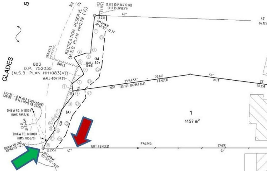
Figure 24: Detail from DP 1232306, showing re-definition of Lot C in DP 380292 (which was a subdivision of original Lot 22), where Mean High Water was adopted, which meant that the side boundary was increased in length by 6.2 m – 2016.
