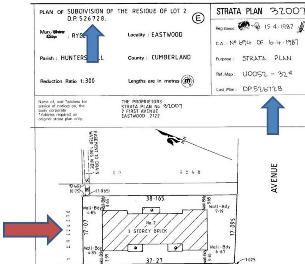
Figure 33: Detail from SP 32007, showing incorrect reference to base Deposited Plan – 1987.
