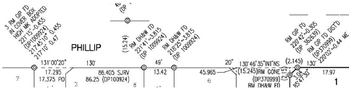
Figure 8: Detail from DP 126124, showing the multiple GI pipes at either end of Phillip Road – 2018.
