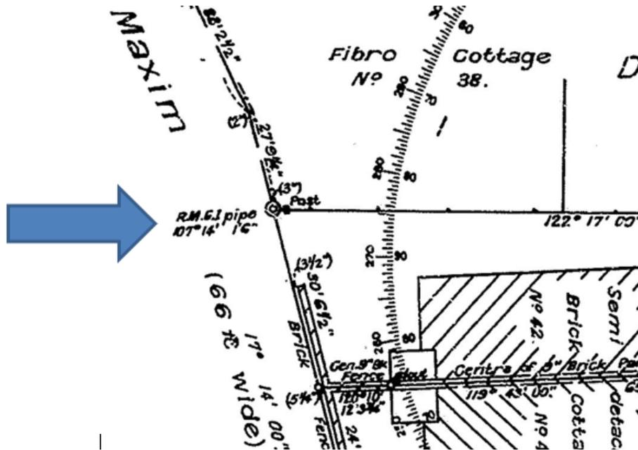
Figure 9: Detail from DP 202784, showing reference mark GI pipe placed at 0.457 m square to the line of the street – November 1960.
