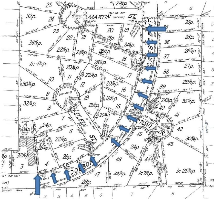
Figure 1: Detail of DP 24598 showing 15 concrete block reference marks defining 12.192 m straights in the road boundary definition, rather than a single arc, which would require just two reference marks – 1951.
