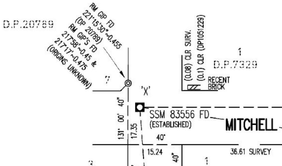
Figure 4: Detail from DP 1246370, showing three GI Pipes at the one corner – 2018.
