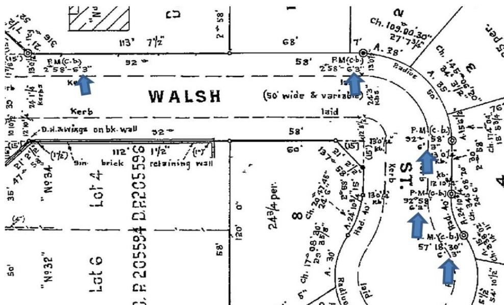
Figure 2: Detail from DP 218164, showing reference marks placed at 6ft 3in – 1962.
