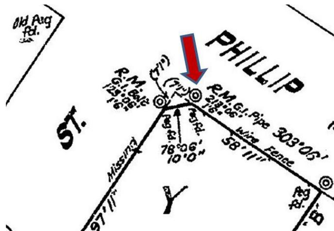
Figure 6: Detail from DP 370999, showing reference mark GI pipe placed at 1ft 6in for the same corner – 1950.
