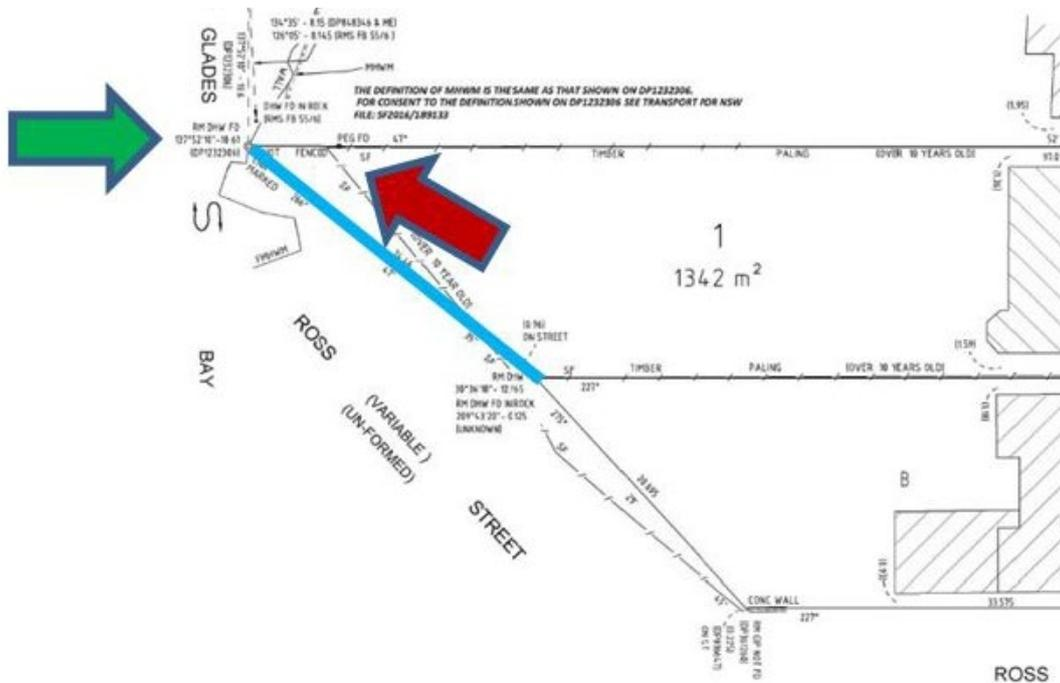
Figure 25: Detail from re-definition DP 1264104, showing that a point contact with the natural boundary has been retained – 2020.
