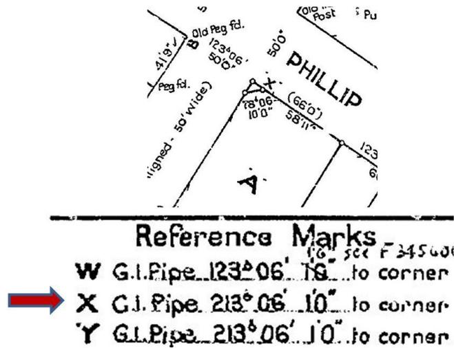
Figure 5: Detail from DP 362639, showing reference mark GI pipe placed at 1ft 0in for corner 'X' – 1944.
