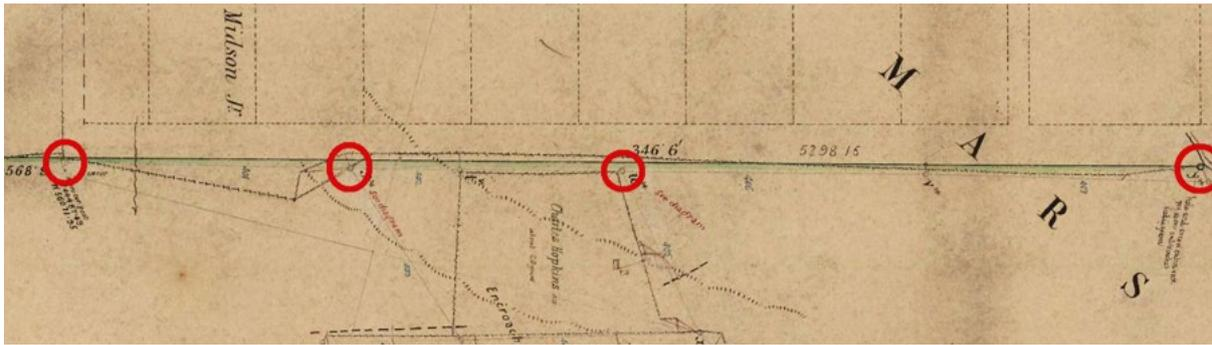
Figure 28: Detail from Crown Plan 15.440 (sheet 4), showing divergence between the traverse lines and the straight-line boundary (green).
