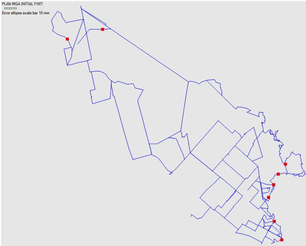
Figure 20: Closed loops in the adjustment with the 8 selected control marks (red) held fixed.
