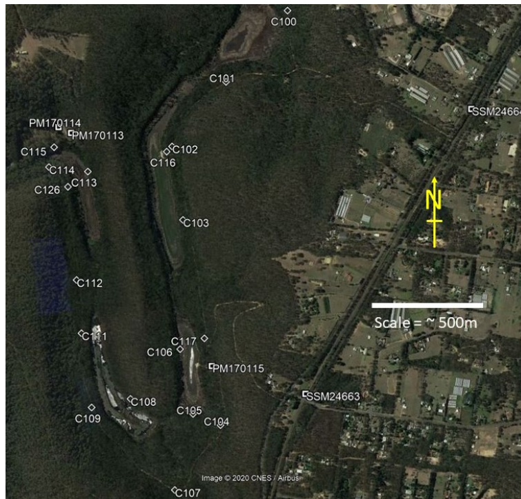
Figure 3: Google Earth overlay of control marks and existing SCIMS control (points C102, C117, C107 and C112 were link points between the adjacent student groups).
