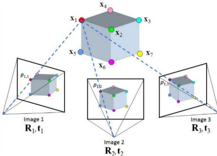
Figure 1: Structure-from-motion process (Yilmaz and Karakus, 2013).
