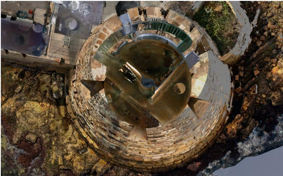
Figure 23: Bottom-up view of Fort Denison 3D reality model, showing interior rooms of tower and external tower walls.
