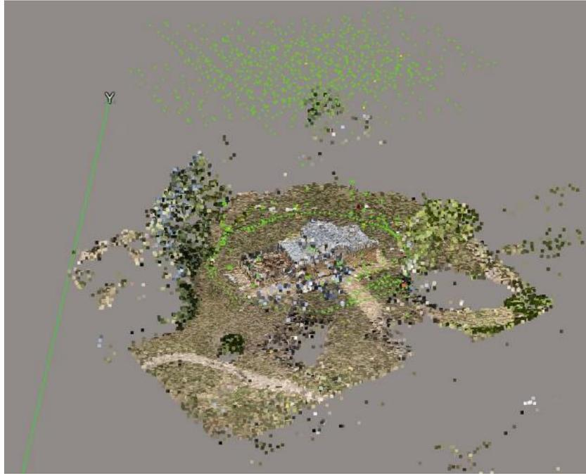
Figure 9: Aerotriangulation results showing computed point cloud and location of manually flown oblique RPAS images, handheld images and nadir and oblique semi-autonomous RPAS capture images.
