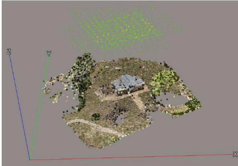
Figure 8: Aerotriangulation results showing computed point cloud and location of nadir and oblique images captured from semi-autonomous RPAS flights.
