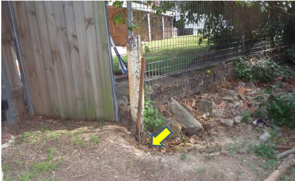
Figure 4: Original broad arrow rock mark found (450 mm deep) at base of white painted steel post.
