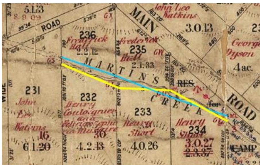
Figure 3: Plan 386.2030 (1881-82) with right lines joining corner marks (yellow) and creek traverse (blue).
