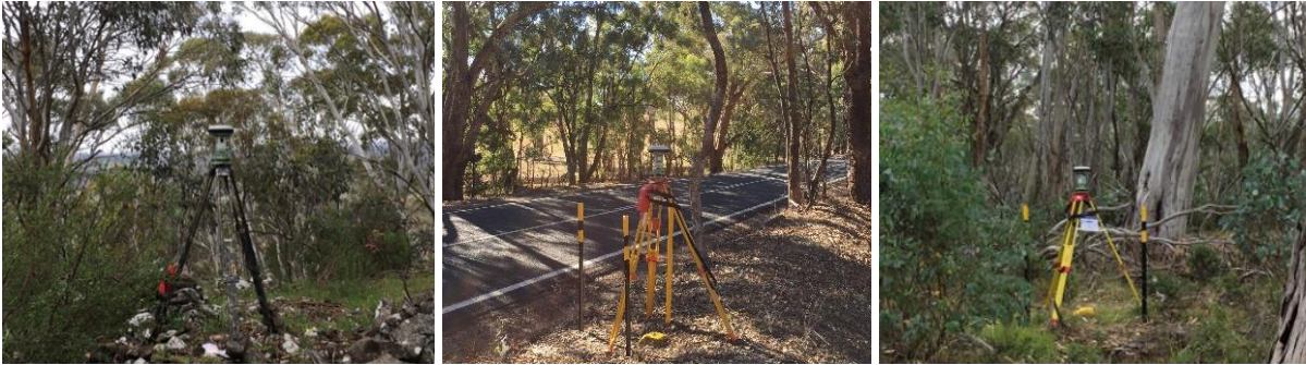
Figure 4: Pushing the boundaries of reasonable sky view conditions in the field: TS486, SS4115, MM3634.
