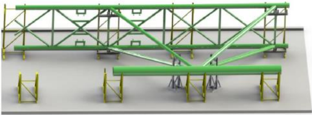
Figure 6: Assembly sequence of nodes/braces into the final jig.
