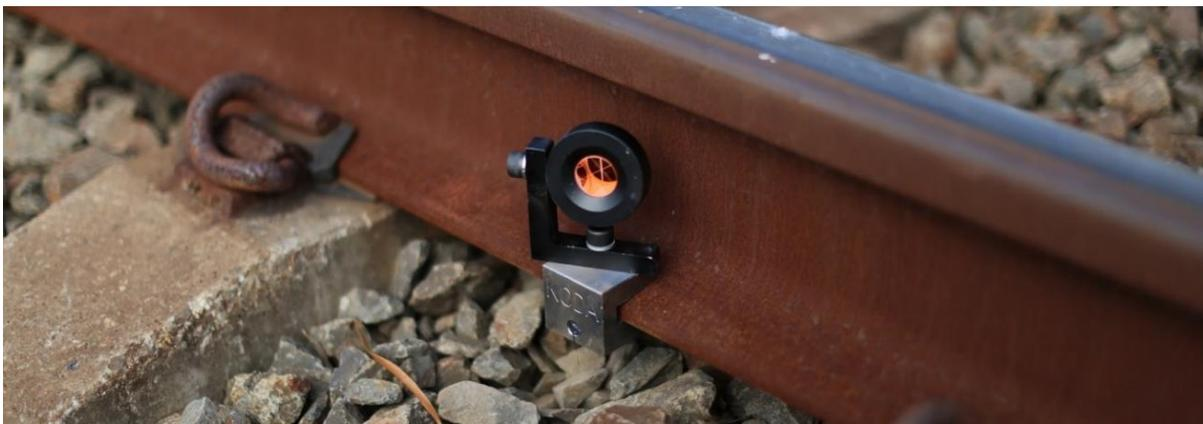
Figure 3: KODABlock track monitoring target.
