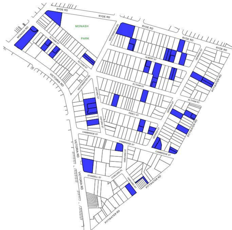
Figure 18: The current cadastre, showing the 50 lots connected to MGA.
