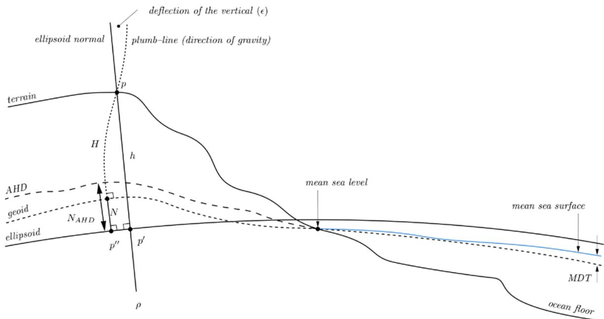
Figure 2: Reference and working surfaces for height in Australia.
