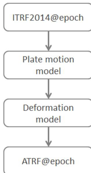
Figure 3: ATRF coordinates computed by applying the secular motion from a plate motion model with the deformation model.
