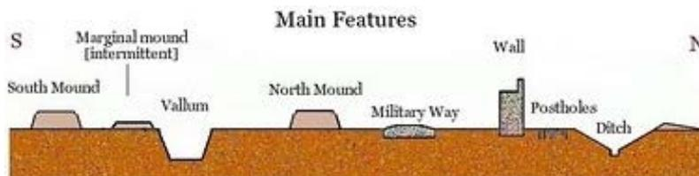
Figure 5: Cross sectional diagram of the Wall construction.
