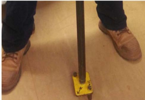
Figure 3: Rail tool on sighting pole.
