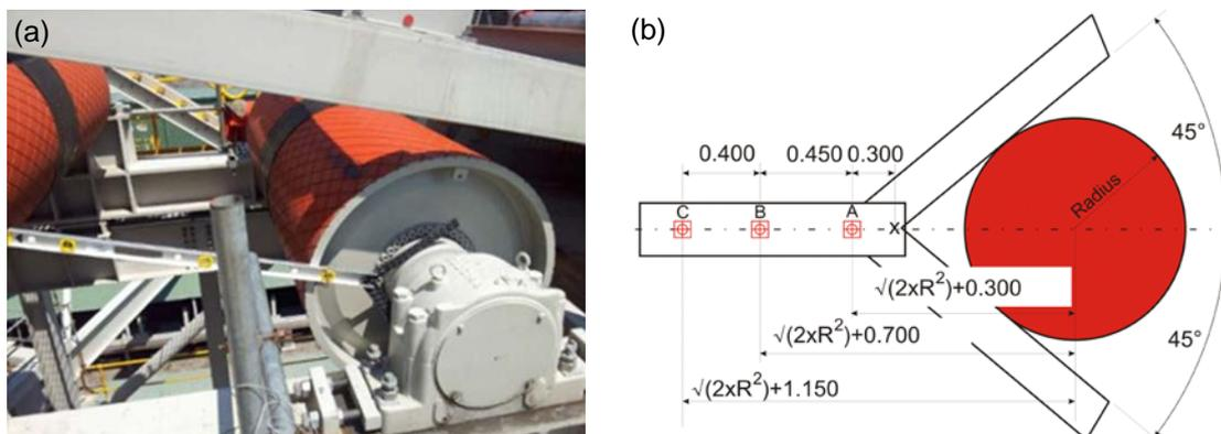
Figure 14: (a) Roller tool in use, and (b) roller tool schematic.
