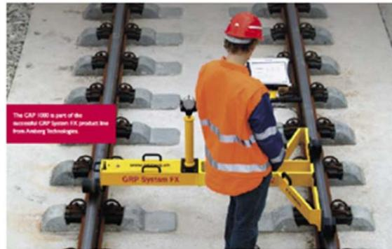
Figure 1: Leica GRP1000.
