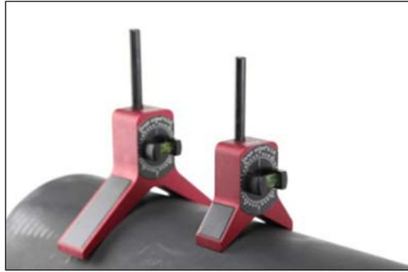
Figure 15: Commercially available flange wizard (Flange Wizard, 2017).
