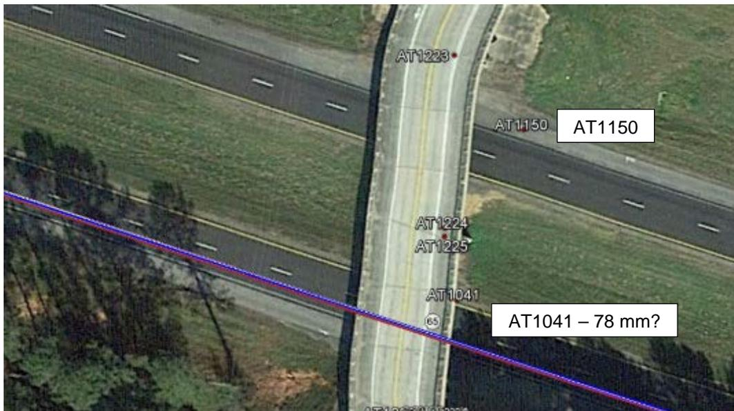
Figure 12: Control coordinate discrepancy.
