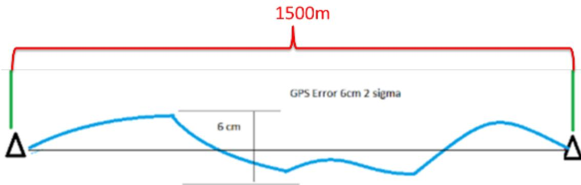
Figure 1: Satellite errors affecting kinematic GNSS.
