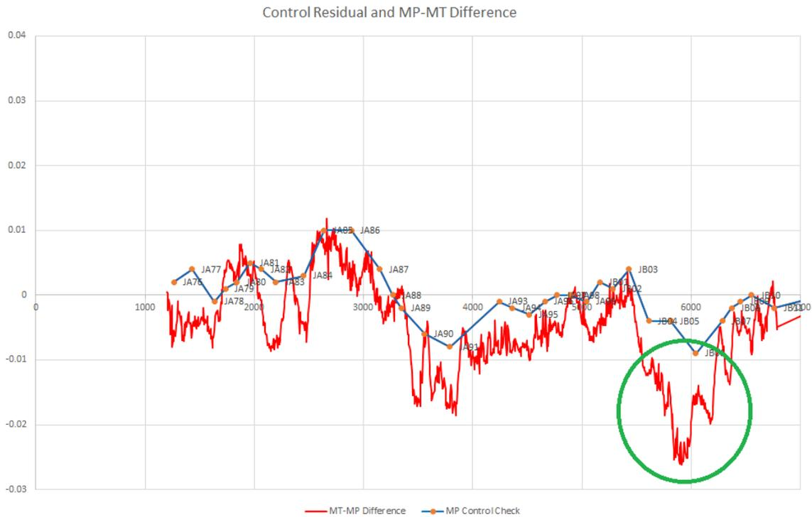
Figure 5: Difference in point cloud 1 (values in metres).
