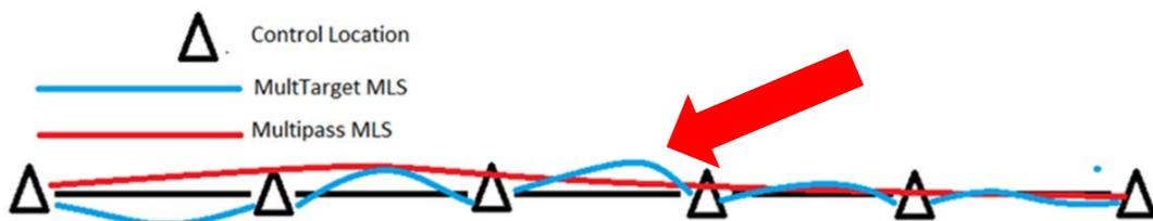
Figure 9: Possible cause of point cloud deviation.
