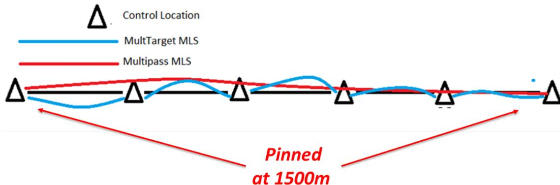
Figure 3: Multi-pass approach compared to multi-target approach.
