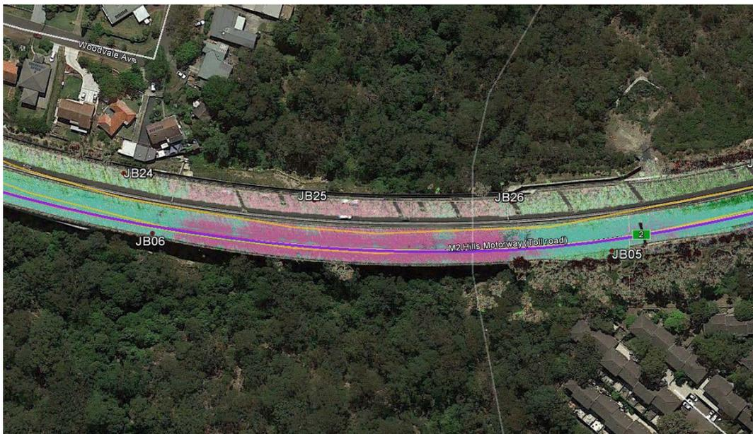
Figure 6: Image of point cloud deviation 1.
