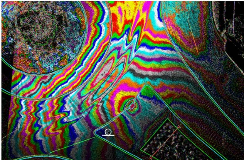
Figure 2: 1 cm contour of a roundabout.
