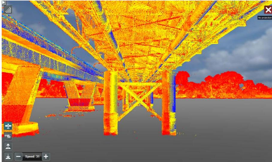
Figure 4: Measurement under the deck of Shoalhaven Bridge.
