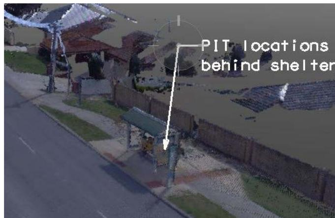
Figure 7: Pit location behind a bus shelter – requires field survey.
