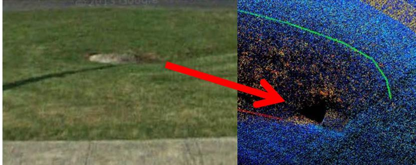
Figure 6: Drainage pipe in imagery and laser scan.
