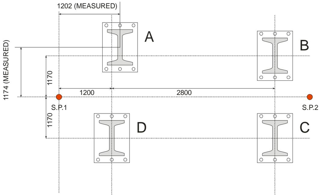
Figure 3: Column measurements.
