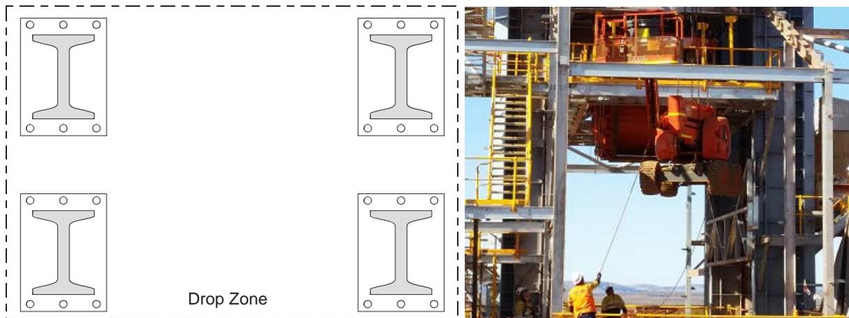
Figure 6: Drop or exclusion zone (left) and drop zone example (right).
