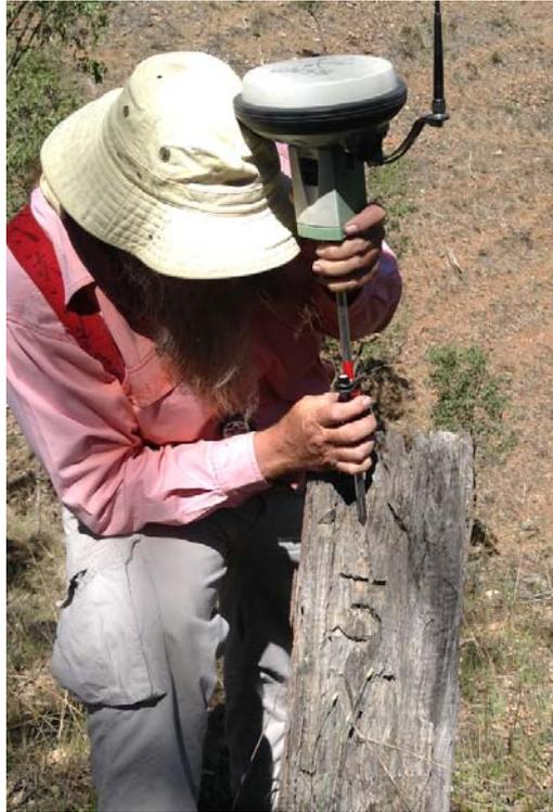
Figure 2: Adaptor for measuring posts.
