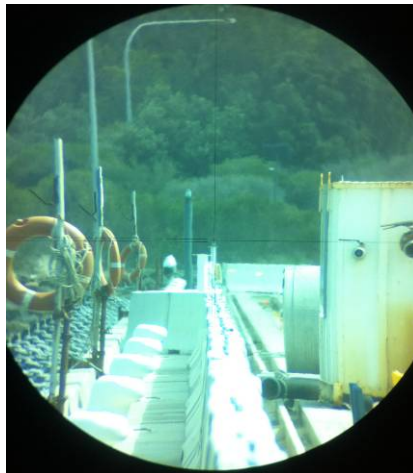
Figure 9: Jersey kerbs reducing effective ground clearance of total station observation.
