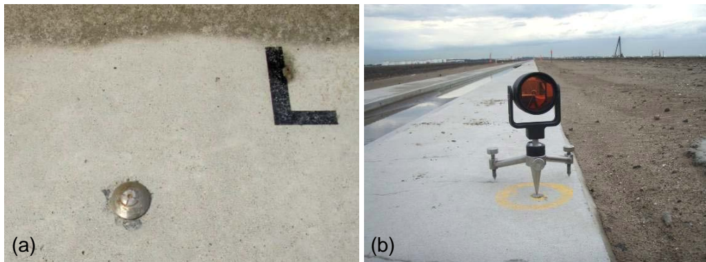
Figure 2: (a) Stainless steel settlement pin in crane rail and (b) prism set up on settlement pin using mini-tripod and mini-pole.
