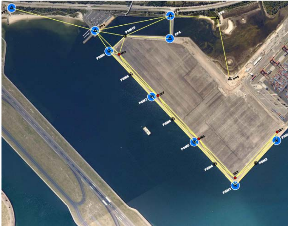
Figure 8: Epoch 4 survey control network showing integrated GNSS and braced-quad configuration.
