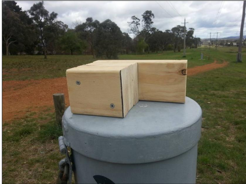
Figure 4: Timber block used to determine the beam dimensions and alignment.
