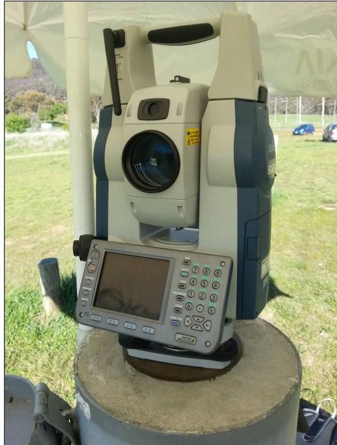
Figure 3: Sokkia SRX3X total station used in the case study.
