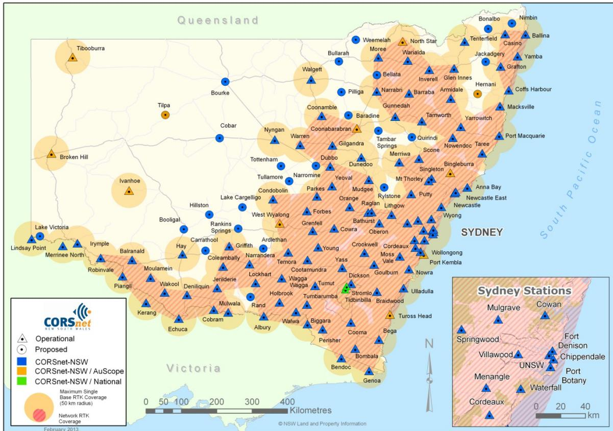
Figure 1: Current coverage of CORSnet-NSW (February 2013).
