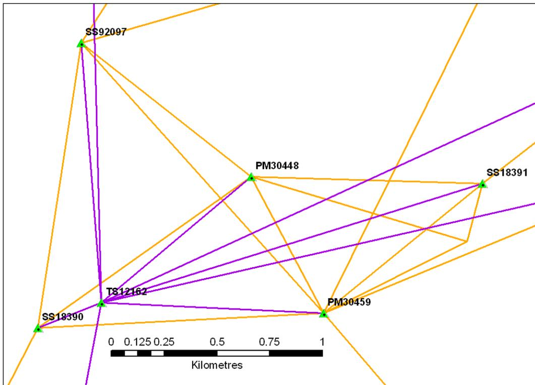
Figure 4: A typical local array network (here for Lockhart CORS), showing the tie survey baselines (purple) along with the existing A1 sub-spine (orange).
