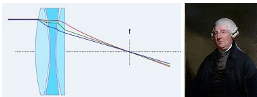
Figure 5: Triple achromatic (or apochromatic) lens (left) and Peter Dollond (Royal Museums Greenwich) (right).
