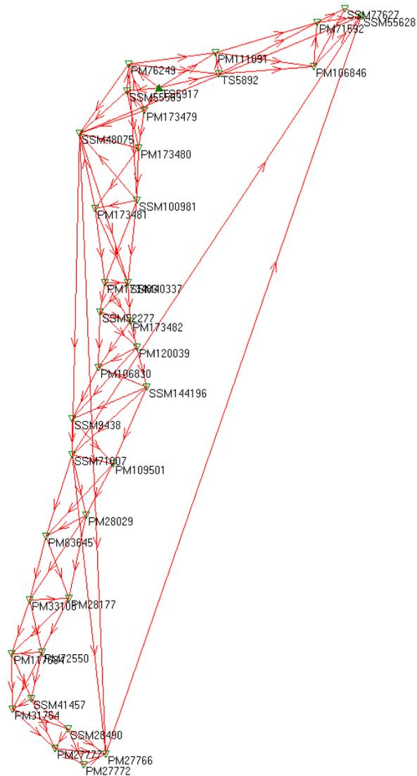
Figure 5: Static GPS control network comprising a system of braced quadrilaterals from Tomago to Stroud Road.
