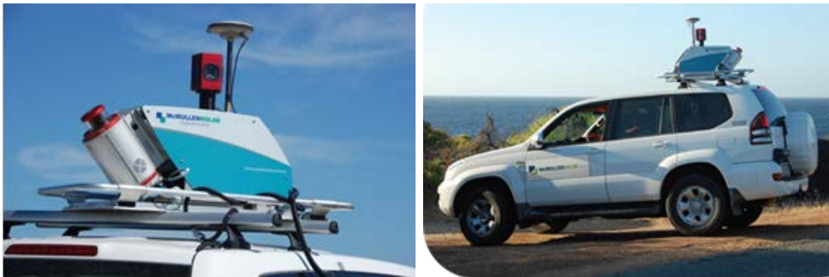
Figure 2: MLS system components and mounting on working vehicle.
