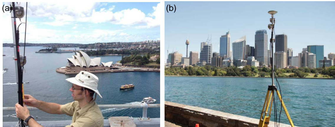
Figure 9: (a) LocataLite atop Sydney Harbour Bridge, and (b) LocataLite near seawall of Botanical Gardens.
