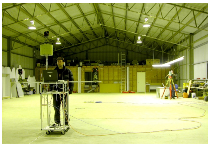
Figure 7: Indoor test site, Locata receiver on trolley and RTS set-up.
