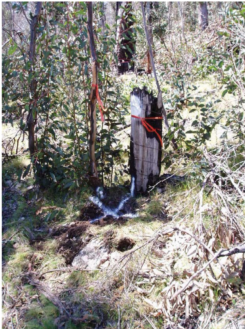
Photo 7: Burnt-out corner post and RMGIP from Peter Cooper's 1957 survey at West Denison
